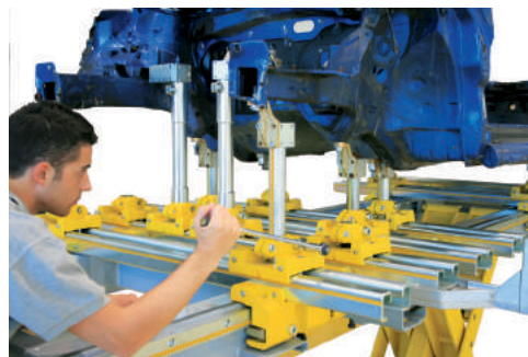
Upward and downward pulling system and possibility to move the cross members with rack and pinion system
