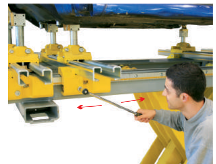
Upward and downward pulling system and possibility to move the cross members with rack and pinion system
